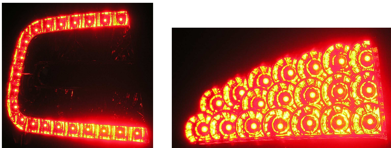
Figure 3: Example of lit appearance of reflector array with direct reflectors.
